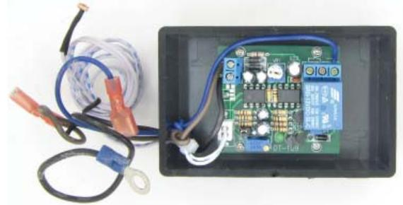
Figure 3. The wired and Boxed Module
