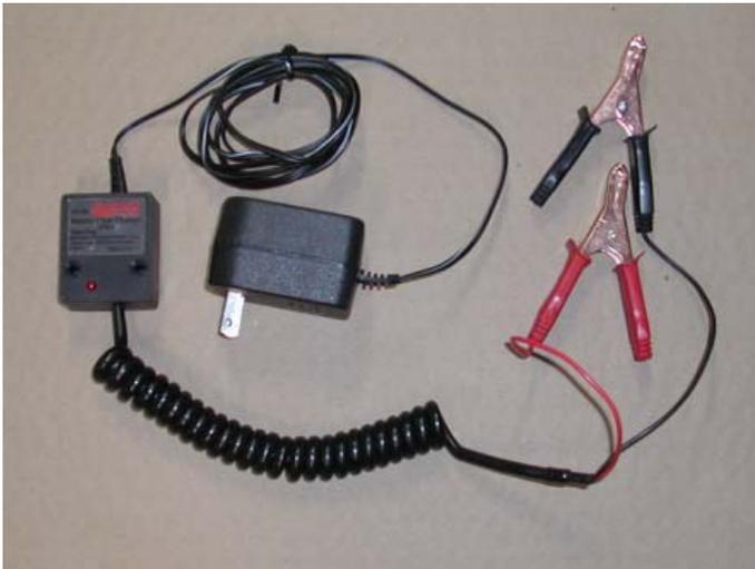
The trickle charger uses a wall-block transformer and an electronic module to regulate the charge rate.
