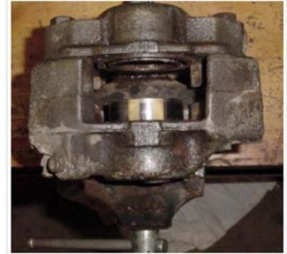
1. Remove bleeder screw and hold piston in that is frozen with a clamp and install a grease fitting in bleeder screw hole. Hand pump grease into it. usually this breaks it free.
