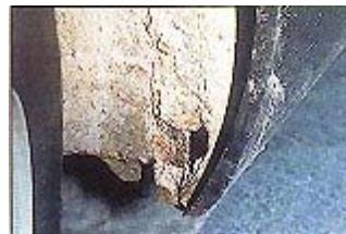
*Rust damage to lower bolt-on splash panel, corrosion may have also spread to the sill sections.*
