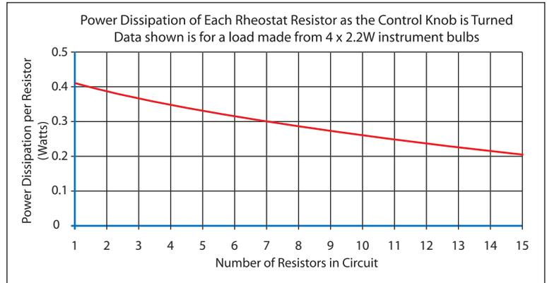
Fig. 5. Power dissipation of rheostat resistors
