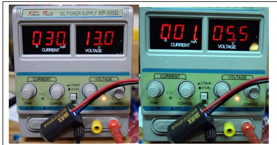
value generally considered to be that where sulfation is a risk. Unlike the ProPulse, when the voltage was reduced, as that of a discharging battery would, it did not switch itself off. Indeed, as the illustration shows, even after the voltage was dropped to as low as 5.5V (right), the Max was still drawing a little current.
