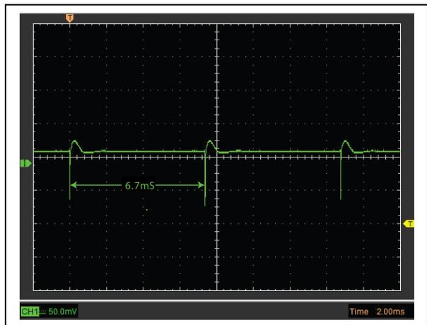
This oscilloscope trace also shows the rate at which the Max pulses are produced, one every 6.7mS, or at a frequency of 150 times per second.
