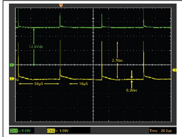
It may be that the small but long battery discharge pulse followed by the quick but large charge pulse of the ProPulse is equally effective at preventing and/or reversing desulfation as newer devices that exhibit both discharge and charge pulses of high magnitude and short duration. There is not enough data available to know for sure.
