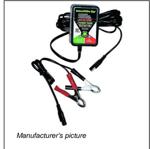
The BatteryMINDER has two LEDs. A red LED indicates that the unit is plugged in to ac power. The green LED indicates that the unit is connected to the battery. This LED is solid green when charging at full output but, when the battery reaches 14.2V, it trips to its 13.4V maintenance voltage whereupon the green LED flashes. A button allows the user to force the BatteryMINDER into maintenance mode if desired. The device also features short-circuit and reverse voltage protection.
