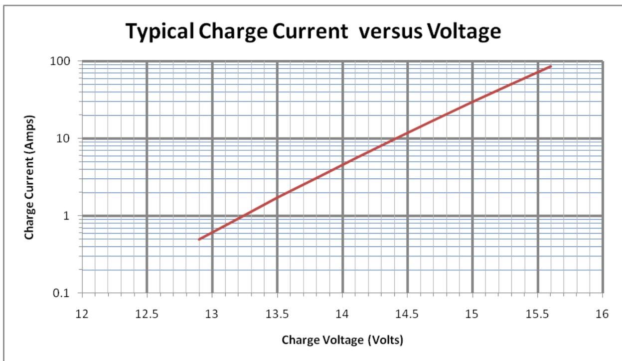
With a normal trickle charge voltage of 13.2V applied, this battery accepts a charge at a little less than 1A. Note how an increase of as little as 1V in charge voltage to 14.2V increases the charge current to 7A while another 1V increase to 15.2V increases the charge current to a whopping 40A. If a desulfator can produce a positive voltage spike of several volts, even for a tiny amount of time, it will result a momentary very large charge current.
