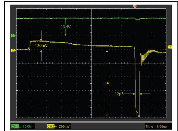
The 1V negative pulse, on the other hand, might be expected to result in a very short discharge pulse of some 80 or so amps.
