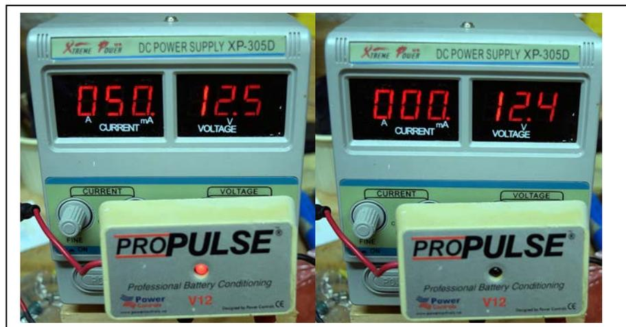
indicates it has lost some capacity. This desulfator still draws a current of 50mA at 12.5V (left) and its own LED indicates that it is still drawing current. However, when the voltage drops to 12.4V (right), the current drawn drops to zero and the LED is no longer illuminated, indicating that the device has switched off. This action prevents the ProPulse from running down the battery with the attending consequences.
