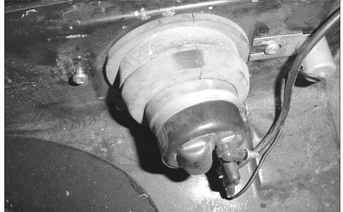
Disconnecting the electrical connections to a fuel pump is easier on some cars than others.
