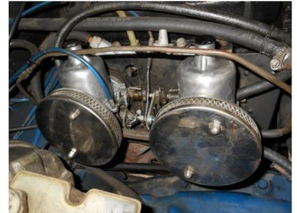
bowl had stuck open (these are HIF carbs). I called Hagerty Insurance to have the car towed from my garage to his shop. He called later, telling me he'd found a small piece of black rubber inside the carburetor's fuel bowl. He planned on replacing the fuel lines between the filter and carburetors, when rebuilding the fuel bowls since they've likely been damaged by ethanol which unfortunately is always present wherever we buy gas today. When
