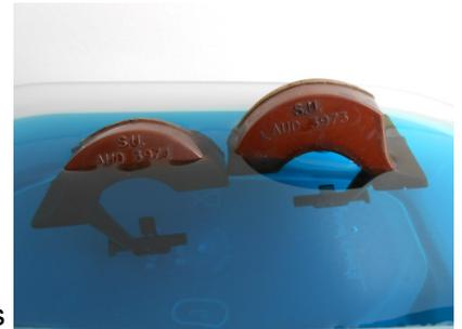
rebuilding the carburetors he discovered another unexpected problem; one of the plastic floats wasn't working properly. Somehow, a small amount of liquid had gotten inside and it was no longer shutting off the fuel (strange since the car had run fine just two days earlier).
