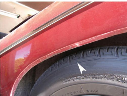
175/70-R14 radial tires I'd had fitted resulted in fouling of the left wheel arch as arrowed in the picture and, knowing of the left offset of the axle, I had put it wholly down
