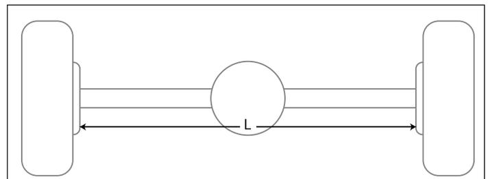
can check yours by running a steel tape measure between the flat areas of the brake back-plates, as shown in the sketch. The exact measurements depend on a plethora of variables and tolerances but for a wire-wheel axle, dimension L should be about  $46\frac{1}{4}$ " and for an axle designed for bolt-on wheels, about 48".
