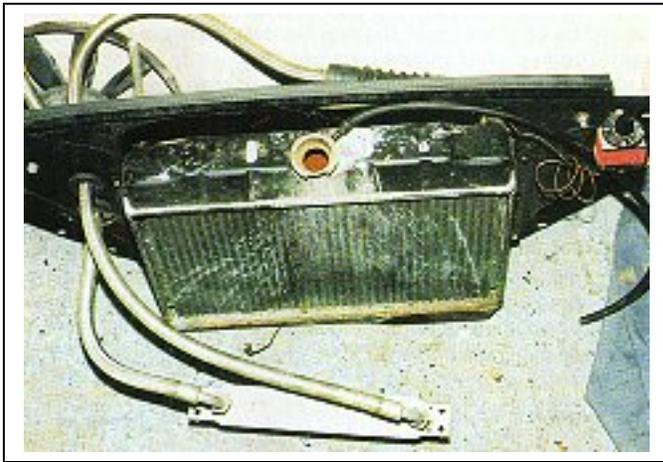
from the block. This will improve access to the main oil cooler hose, which can now also be removed. If there electrical oil pressure gauge, remove the wire from the sender. The four 7/16" A/F bolts that retain the oil cooler should now be removed
