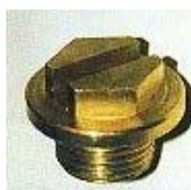
British Standard Pipe Thread (BSP), sometimes found on sump and gearbox plugs, which has a tapered form so as to 'seal' the hole when tight. They are basically Whitworth 55 degree form but are nominated by the bore of the pipe. i.e. 1/4" BSP is about 0.528" O/D and 20 TPI. This is why 3/16 Whit wrenches often fit brake pipe unions. BSP threads are were adopted by the ISO-metric system so will be found even on
