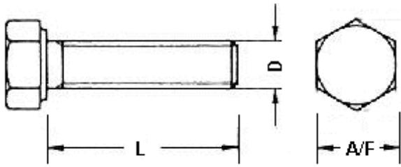
F. For instance, as shown in the first table below, a 5/16" UNF threaded bolt has a 1/2" A/F head.
