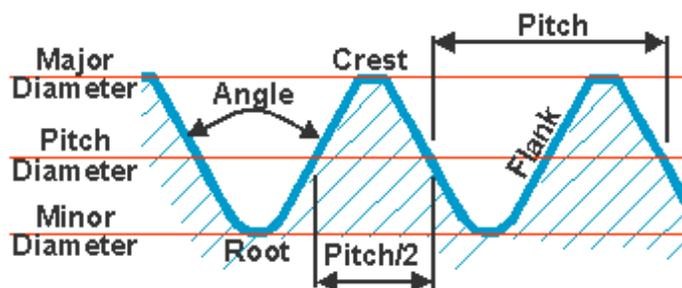
measured in turns per inch or centimeter. Whitworth's form was so successful that vestiges of it still appear in many current types. To augment Whitworth's BSW thread a fine thread version called BSF was introduced in 1908. British Association (BA) threads were standardized in the early 1920's for sizes smaller than 1/4".
