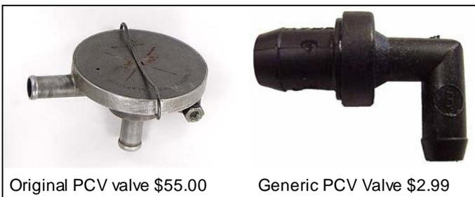
Inspecting the PCV valve showed its diaphragm to have a split in it, so, rather than continue venting engine gases to the environment I replaced that for about \$5.
