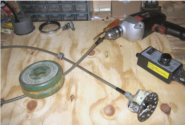
this way, the indicating needle, mounted on the same shaft as the cup, reads higher as the speed increases.
