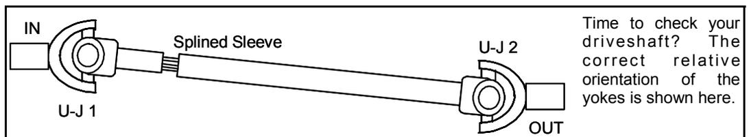
Time to check your driveshaft? The correct relative orientation of the yokes is shown here.
